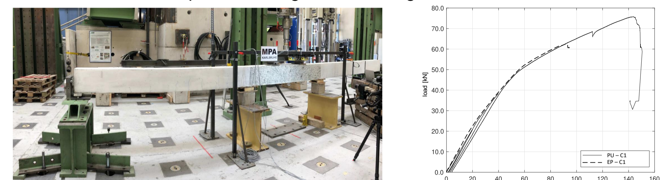
Figure 4: strengthened bending beam in four-point bending test (left) and load-deflection-curves (right)
